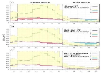
Figure 5. Change in the Selenga river flow under regulation of Shuren HPP (a) Egiin-Gol HPP (b) HPP of Orkhon-Gobi water diversion system (c) at Naushki station for 99% of flow availability
