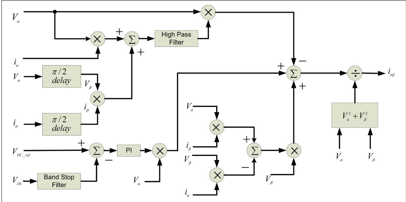
Figure 1. Improved controller schema for bridgeless PFC rectifier.
