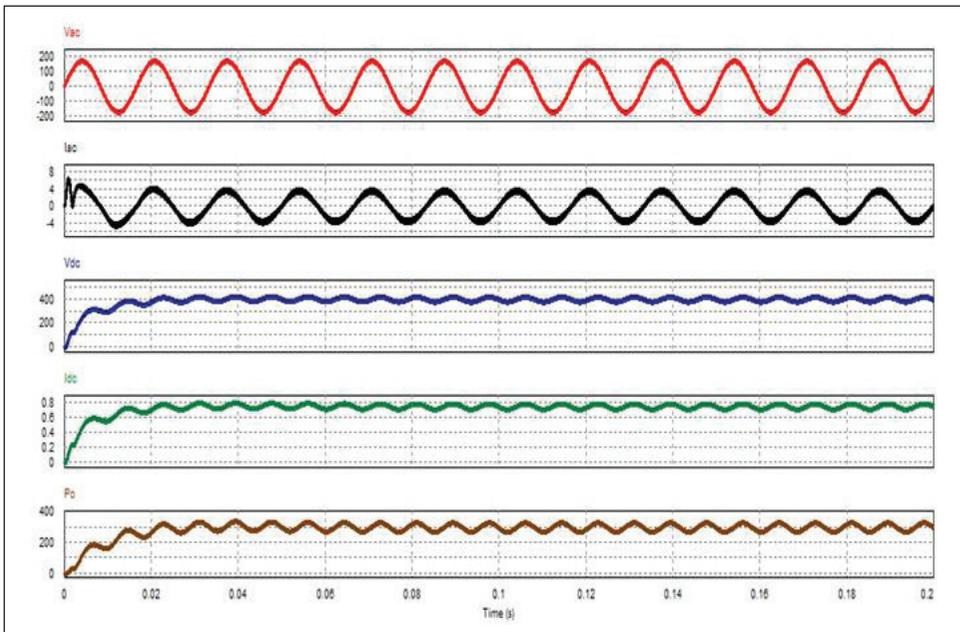
**Figure 5.** The transient input voltage, input current, output voltage, output current and output power for 300W BBPFC rectifier with average current control.
