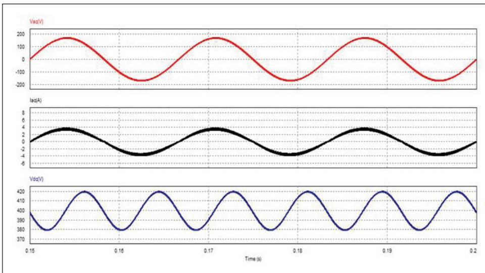
**Figure 6.** The input voltage and current, output voltage waveforms for 300W BBPFC rectifier with average current control (PF 0.9894, THD %5.51).
