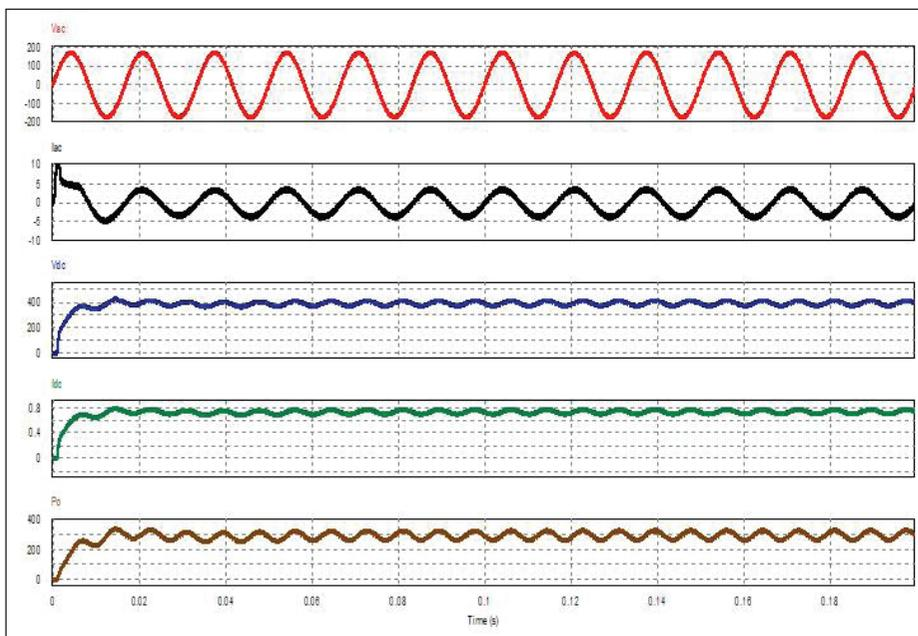
Figure 8. The transient signals for 300W BBPFC rectifier with improved  $pq$  controller.
