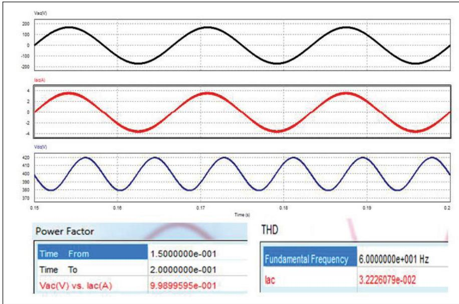
**Figure 9.** The input voltage and current, output voltage waveforms for 300W BBPFC rectifier with improved  $pq$  controller (PF 0.9989, THD %3.22).
