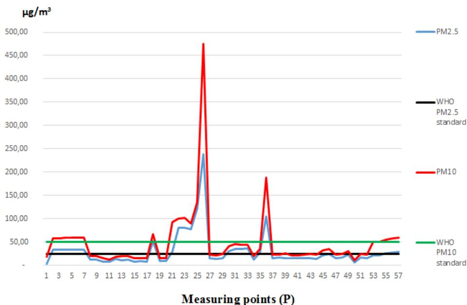
**Figure 3.** PM<sub>10</sub> and PM<sub>2.5</sub> indoor measurement values
