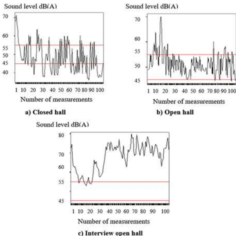
**Figure 5.** Noise measurement values in a. Open hall, b. Closed hall, c. Interview time the open hall
