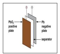
Figure. 1. Chemistry and principal components of a lead-acid battery.
