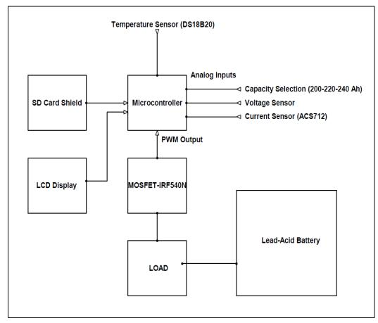
Figure. 2. Hardware diagram
