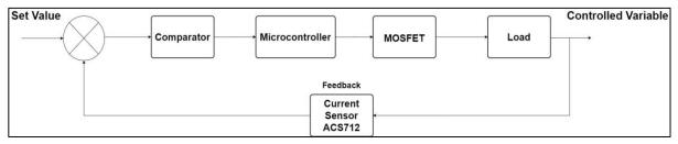
Figure. 3. Block diagram of current control
