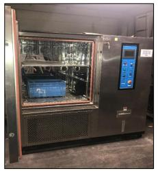
Fig. 6. The battery in the test chamber
