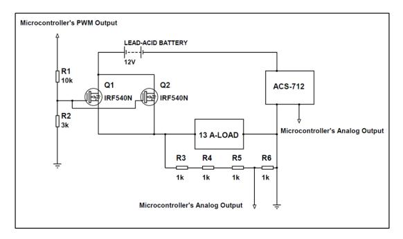
Figure. 5. Battery capacity tester circuit diagram
