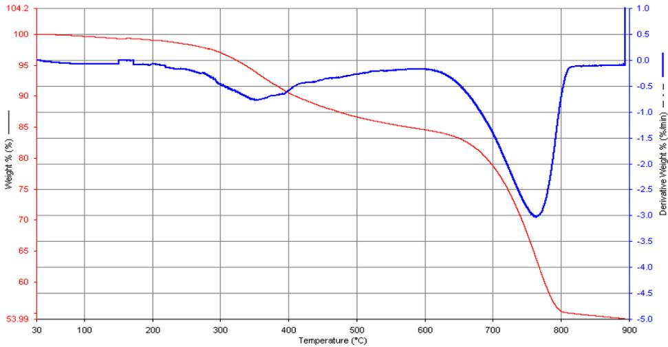
**Fig. 8** DTA /TGA pattern of developed brake with 125 µm periwinkle shell particles
