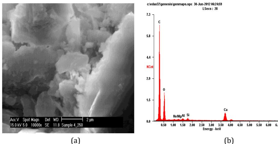
**Fig. 4** SEM (a) and EDS (b) microstructure of developed brake pad with 125 μm periwinkle shell particles
