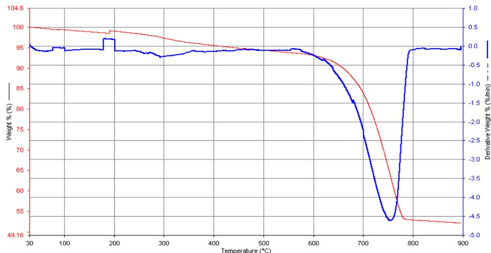
**Fig. 7** DTA /TGA pattern of periwinkle shell particles
