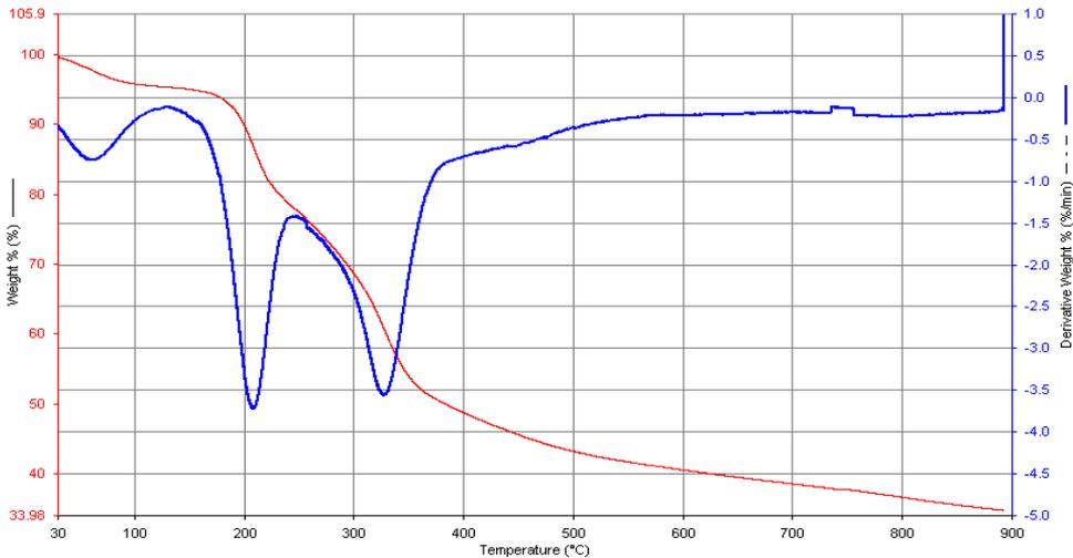
**Fig. 9** DTA /TGA pattern of developed brake with 710 µm periwinkle shell particles
