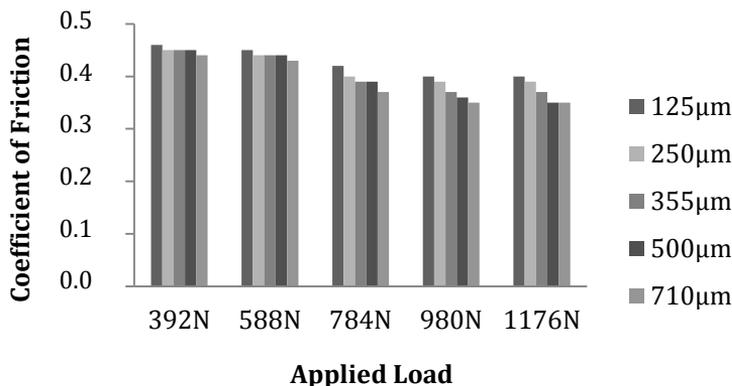
**Fig. 6** Coefficient of friction at varying load at constant speed and time at 250°
