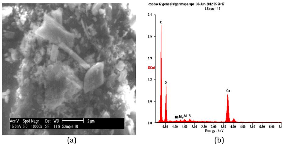
**Fig. 3** SEM (a) and EDS (b) microstructure of developed brake pad with 710 μm periwinkle shell particles
