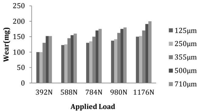
**Fig. 5** Wear (mg) at varying load at constant speed 2.4 m/s, time 45 min at 250°C
