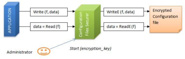
Fig. 3. Secured access to configuration files
