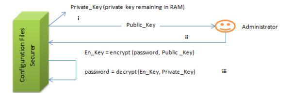
Fig. 4. Starting security module using asymmetric encryption
