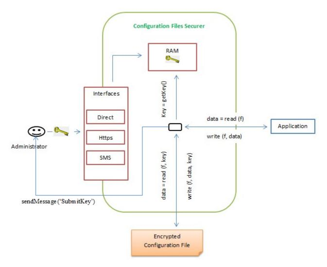
Fig. 6. Internal Schema of the security component
