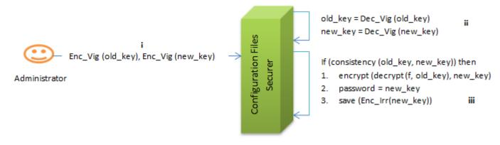
Fig. 5. Starting security module using one-time password
