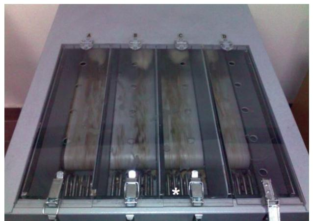
**Fig. 1.** Computerized and motorized treadmill with rats running. Asterisk (\*) shows shock grid, to keep rats running and to record penalty points. [Color figure can be viewed in the online issue, which is available at [www.aott.org.tr](http://www.aott.org.tr)]
