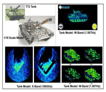
Fig.2. THz Imaging of Tank Model (Goyette, 2003)
