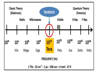
Fig.1 THz in Electromagnetic Spectrum (Zomega, 2012).
