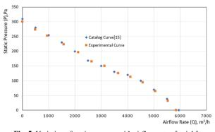
Fig. 5. Variation of static pressure with airflow rate of axial fan
