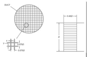
Fig. 2. Cell straightener geometry and dimensions [14]
