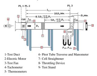
Fig. 1. Axial fan experimental set-up [14]
