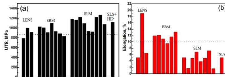
Fig. 2. a) UTS and b) Elongation of Ti64 processed by various AM techniques [96].
