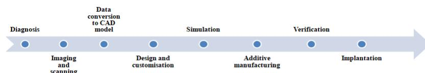
**Fig. 1.** Steps of additive manufacturing process for implants.
