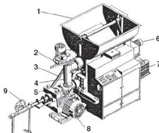
Figure 3. Briquette press (1. hopper crushed straw (sawdust) with spiral discharger, 2. transmission of electromotor for vertical spiral feeder, 3. V-belt of balance wheel for crank mechanism, 4. vertical bailer of straw for presser, 5. pressure regulator, 6. electromotor for discharging spiral conveyor, 7. condenser of cooling unit, 8. electromotor of presser, 9. counter for produced briquettes (length))
