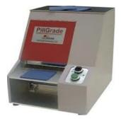
Figure 2. a) Martindale pilling and abrasion tester b) Lissajous movement curve c) PillGrade objective pilling evaluation system
