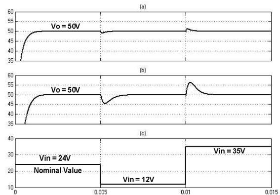
Figure 6. Simulation Results for the Controlled Boost Converter's output response under input voltage variations. (a) LQR Method. (b) Pole Placement Method. (c) Input Voltage
