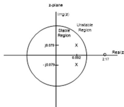
Figure 2. Boost Converter's pole and zero locations in discrete-time domain
