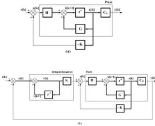
Figure 3. (a) Plant with state feedback, (b) Basic state-feedback with integral actuation
