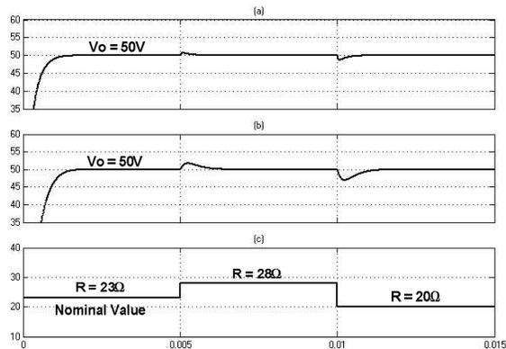
Figure 7. Simulation Results for the Controlled Boost Converter's output response under load variations. (a) LQR Method. (b) Pole Placement Method. (c) Load
