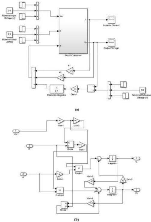
Figure 4. (a) Simulink Model of the controlled Boost Converter. (b) The constructed Boost Converter block in Simulink Model.
