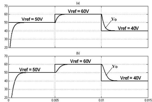
Figure 5. Simulation Results for the Controlled Boost Converter's output response under reference voltage variations. (a) LQR Method. (b) Pole Placement Method.
