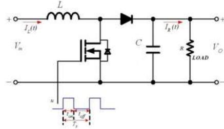
Figure 1. Basic circuit of Boost Converter
