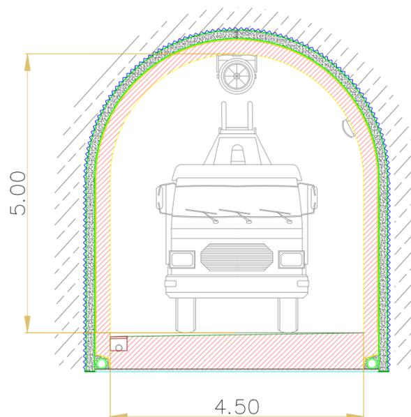
**Figure 2.** Security tunnel type section.
