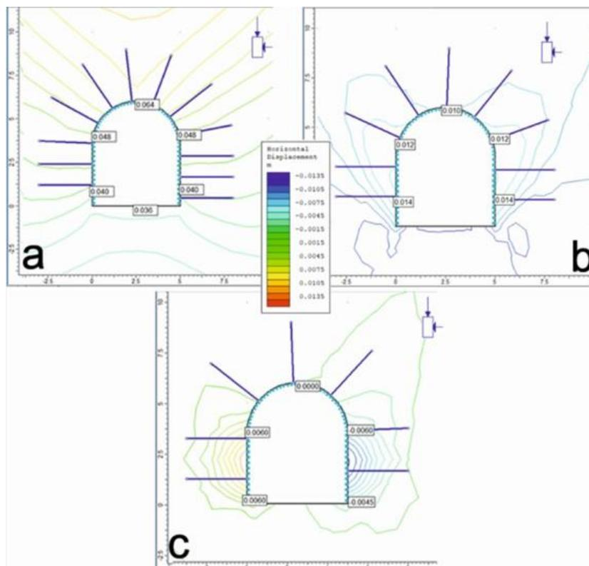
**Figure 5.** Numerical analysis with the Phase program total displacement amounts (a: Porsuk formation b: weathered Bozüyük Granitoid, c: Bozüyük Granitoid)
