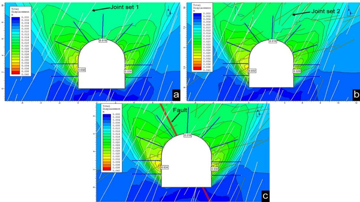
Figure 9. Bozüyük Granitoid region Deformation data of the third region evaluated by numerical analysis (a: Analysis with 1st discontinuity set added, b: Analysis with 1st and 2nd discontinuity set added, c: Fault, 1st and 2nd discontinuity set added analysis)
