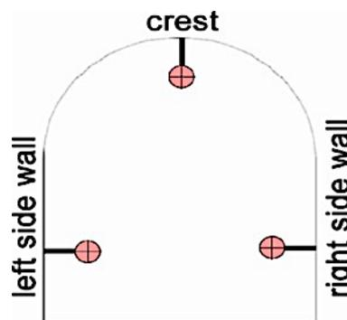
**Figure 6.** Tunnel deformation measurement points.
