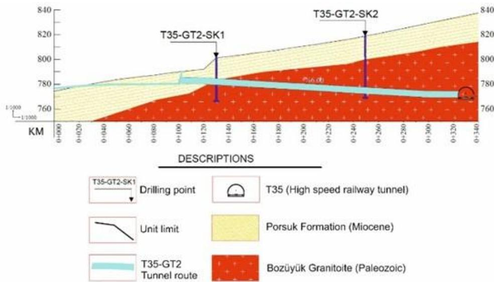
**Figure 3.** Geological map of T35-GT2 tunnel direction.
