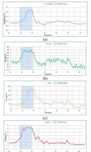
**Fig.8.** Air Quality Data of Laundering Activity a) Humidity, b) CO<sub>2</sub>, c) NO<sub>2</sub>, d) CO
