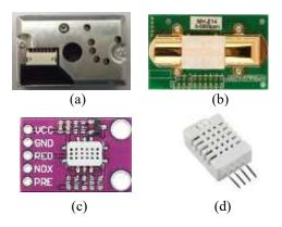
**Fig. 2.** The sensor array used in the proposed e-nose system; a) GP2Y1010AU, b) MH-Z14, c) MICS-4514, d) DHT22.
