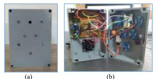
**Fig. 3.** IoT based e-nose measurement system a) Outer view, b) Interior view.
