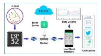
Fig.1. Structure of the proposed IoT-based measurement system.
