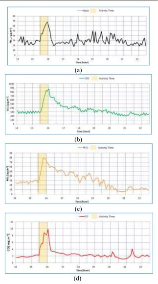
**Fig.7.** Air Quality Data of Cooking Activity a) PM<sub>10</sub>, b) CO<sub>2</sub>, c) NO<sub>2</sub>, d) CO
