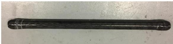
Figure 4. Produced composite shaft.
