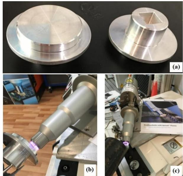
Figure 5. (a) Torsion test fixture apparatuses, (b) plasma application on fixture, (c) plasma application on specimen
