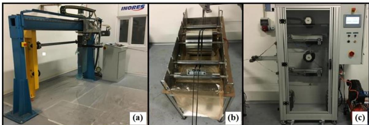
Figure 2. (a) Filament winding machine, (b) resin bath, (c) tension cabinet
