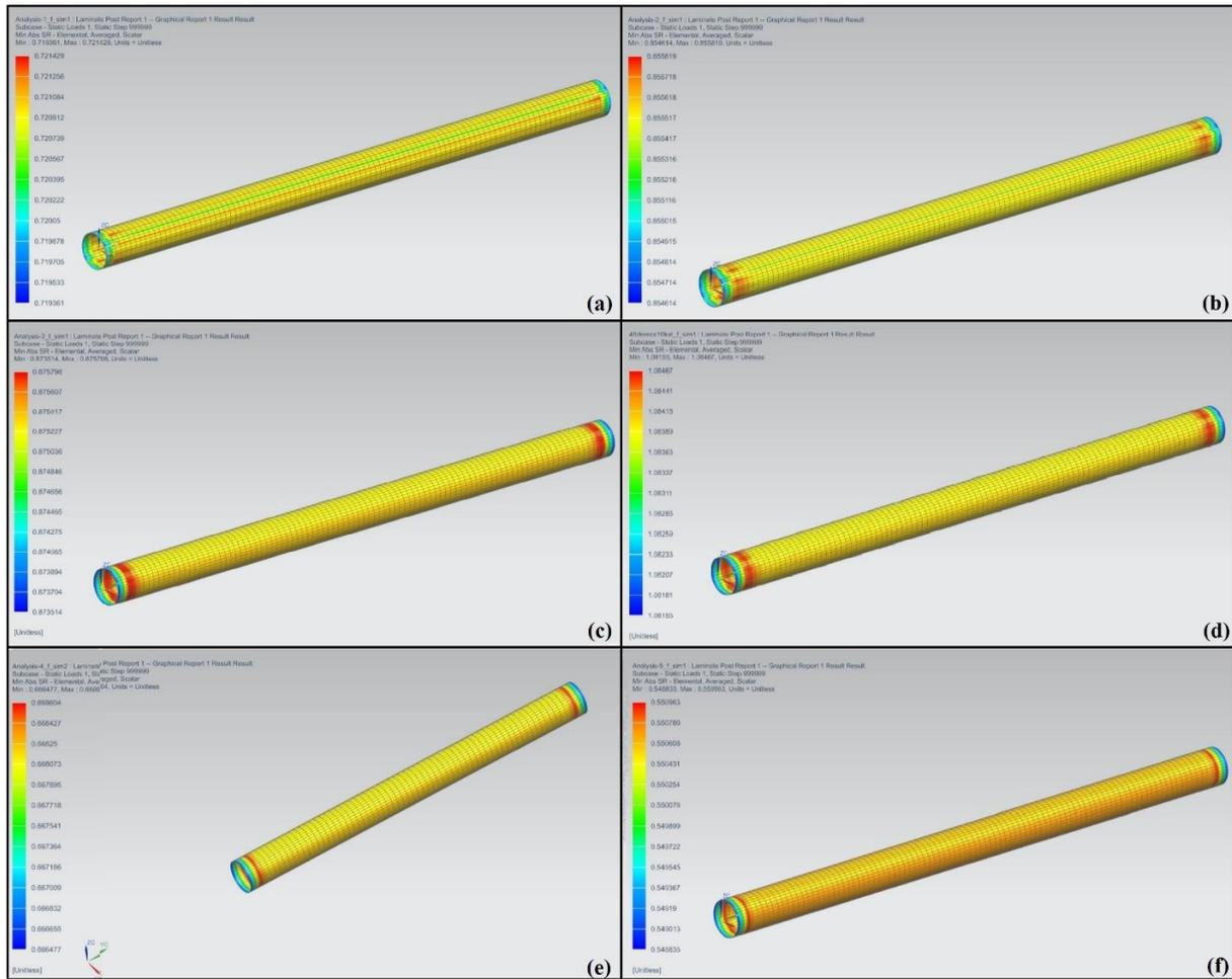
**Figure 6.** Torsion Analysis: (a) 8 layers with +/- 15, (b) 8 layers with +/- 30, (c) 8 layers with +/- 45, (d) 10 layers with +/- 45, (e) 8 layers with +/- 60, (f) 8 layers with +/- 75.
