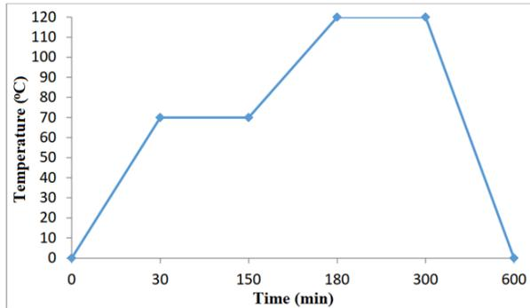
Figure 3. Temperature – time graph of the curing process
