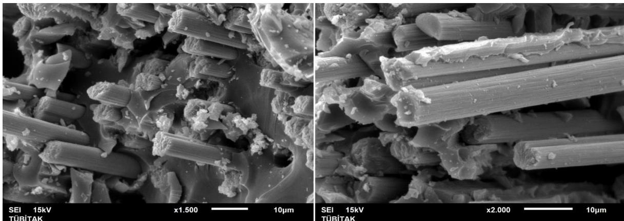
**Figure 8.** SEM images of fracture surface
