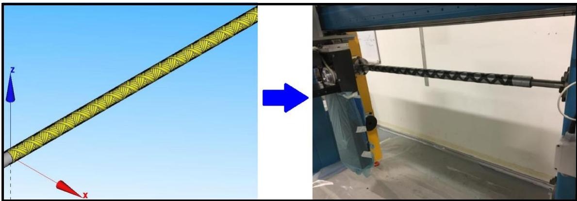
**Figure.** Modelling and production of composite drive shaft
