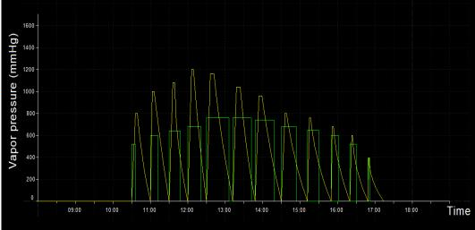
Fig. 9. Vapour pressure in sudden evaporation unit.
