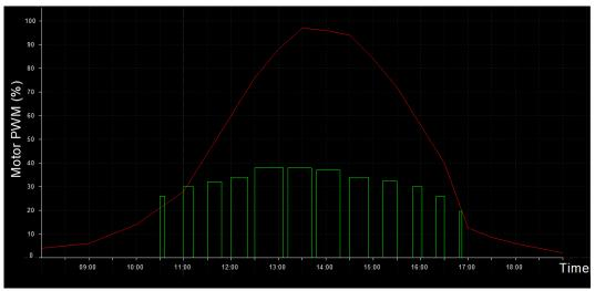
Fig.8. Sea water pump cycle
