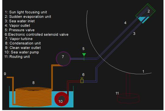
Fig. 5. Diagram of prototype system.
