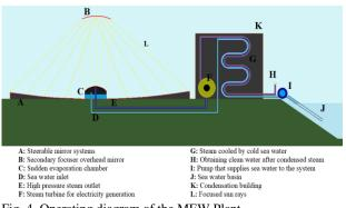
Fig. 4. Operating diagram of the MEW Plant
