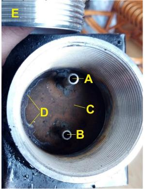
A: Vapor outlet B: Sea water inlet C: The area where sun's rays focused D: Collected minerals residues E: Sudden evaporation unit cover
