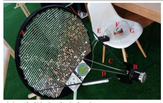
**A:** Array of multiple mirrors focusing the sun's rays **B:** Sudden evaporation chamber
