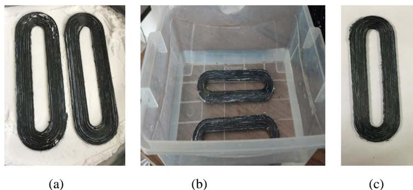
Figure 3. Preparation of CFRTP samples for heat treatment; a) Re-melting in the salt sample, b) Microwave sample, and c) Oven sample.
