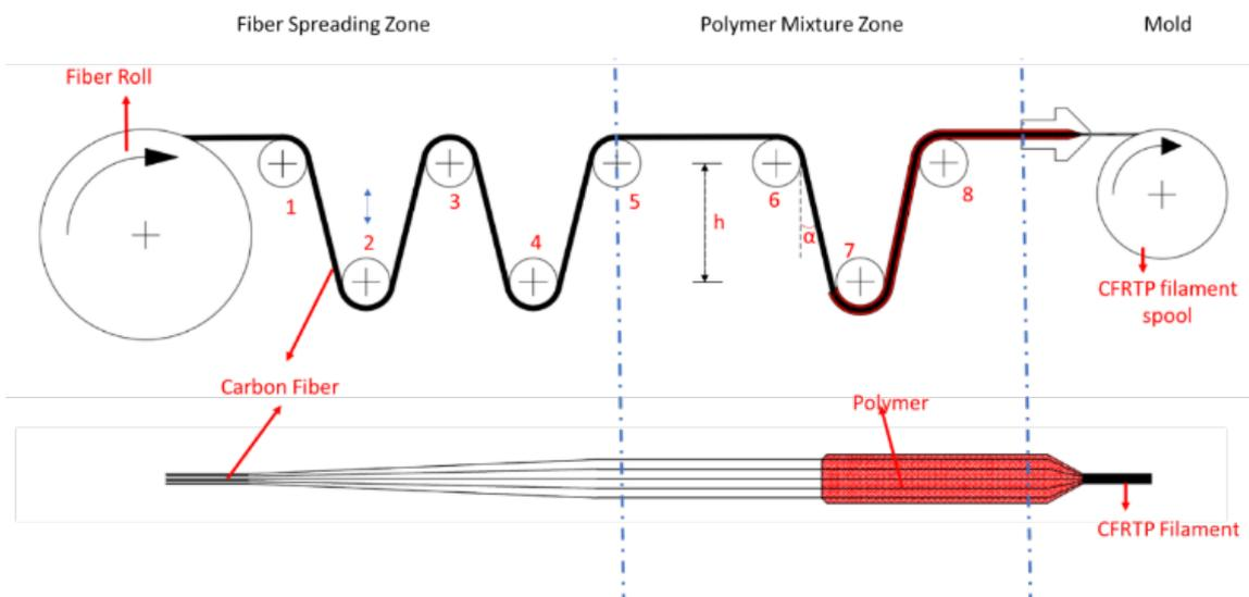
Figure 1. The schematic image of the production line [20]
