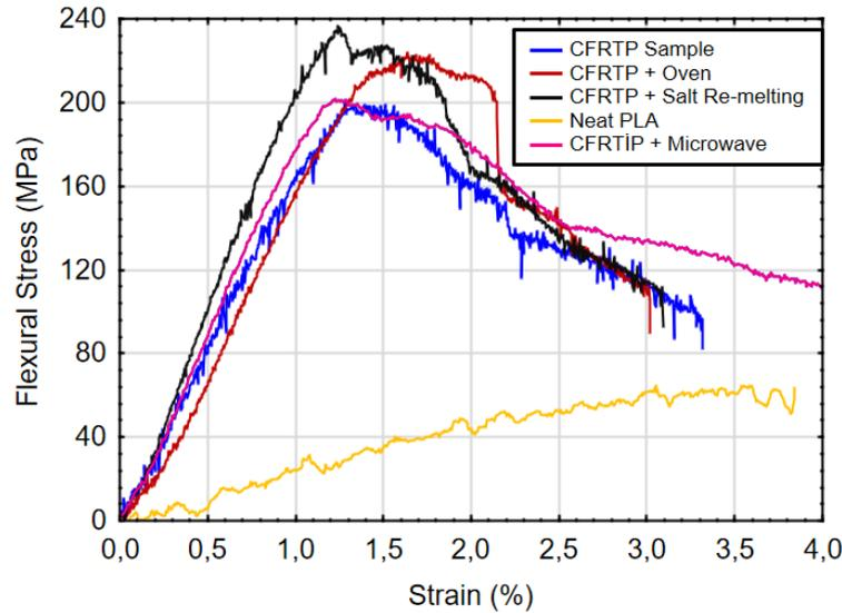
Figure 5. Three-point bending stress-strain curves of CFRTIP samples
