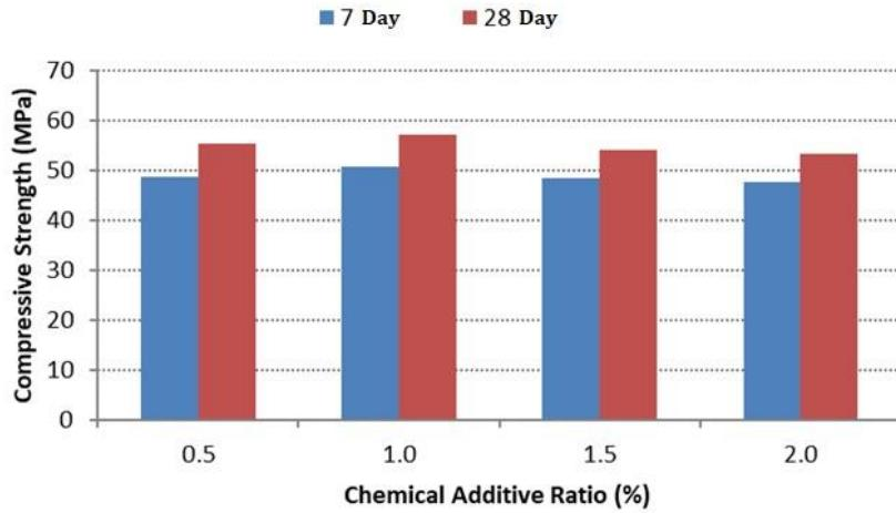
**Figure 4.** Compressive strength values of concrete samples
