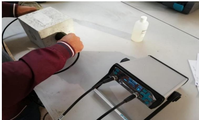
**Figure 2.** Ultrasonic transmission rate determination
