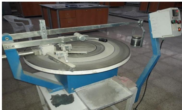
**Figure 1.** Böhme experimental setup
