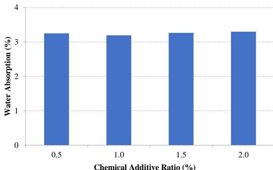
**Figure 6.** Water absorption percentages of concrete samples
