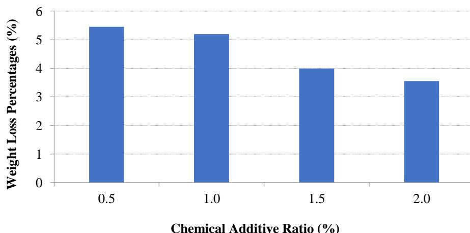
**Figure 5.** Böhme weight loss values of concrete samples
