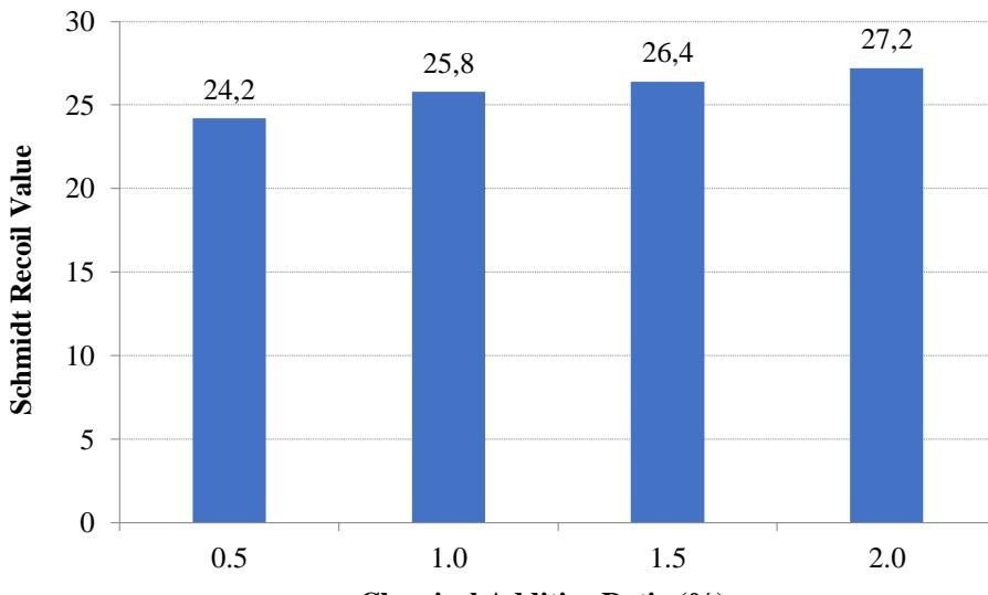
**Figure 9.** Schmidt hammer readings of samples
