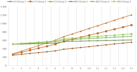
Figure 3. CV and BEV lifetime cost comparison, Scenario 1, thousand dollars
