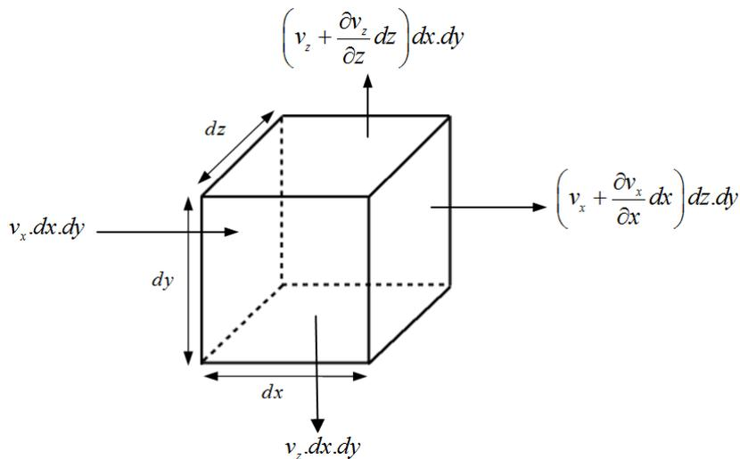
Fig. 1. Flow in point A
