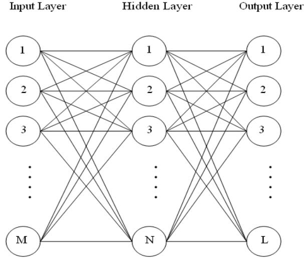
Fig. 3. Schematic diagram of typical MLFF neural network
