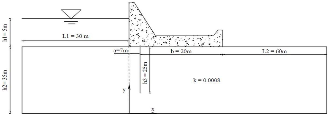
Fig. 2. Characteristics of considered diversion dam
