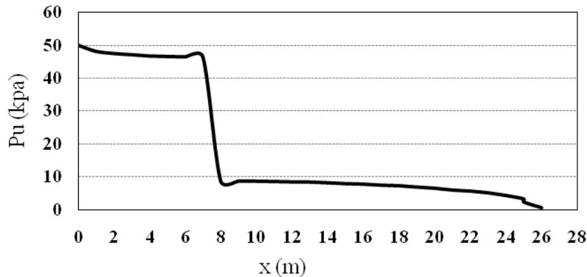
Fig. 5. uplift pressure under the diversion dam
