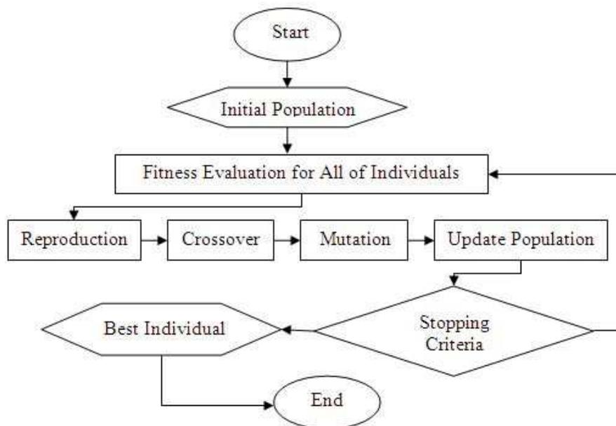
Fig. 4. Flowchart of basic genetic algorithm
