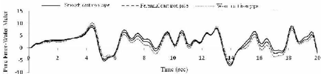
Fig. 3. Differences between water head values obtained in the two mentioned cases versus time at end of the pipe considering the pipe material
