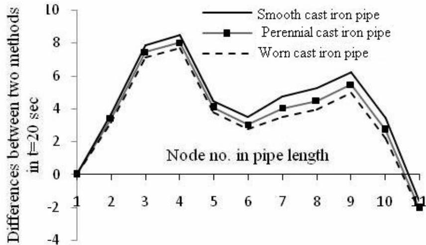
Figs. 9. Changes in water head values obtained in the two mentioned cases along the pipe at t = 20 s
