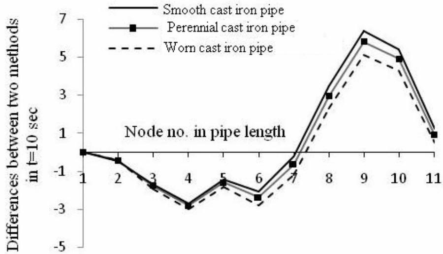
Figs. 8. Changes in water head values obtained in the two mentioned cases along the pipe at t = 10 sec
