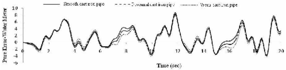
Fig. 5. Differences between water head values obtained in the two mentioned cases versus time in middle of the pipe considering the pipe material
