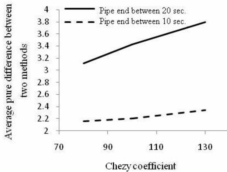
Fig. 11. Mean absolute value of the difference at end part and middle of the pipe versus Chezy coefficient
