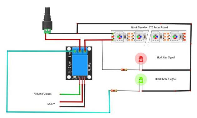
**Figure 10.** The connections of the signals on the line where the train is moving and indicating whether the blocks on the line are occupied or empty.
