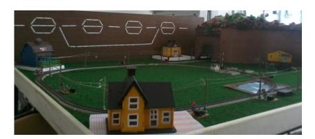
Figure 7. Hardware structure of the designed CTC prototype.
