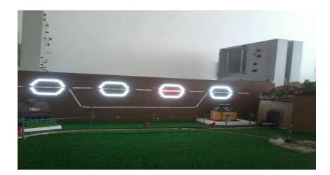
Figure 11. Monitoring of train location (red colour strip led) on CTC board
