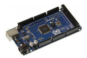
Figure 3. Arduino Mega
