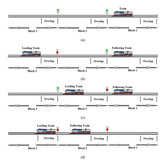
Figure 1. Fixed block system in railways
