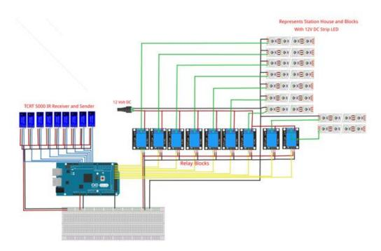
Figure 9. Implemented circuit of "Monitoring of train location system" prepared by using Fritzing program.
