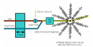
Parallel Flow Injection multichanell analyzer for Olive Oil Peroxide Value determination.
