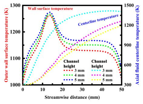
**Figure 12.** Temperature profiles along the outer wall surface of the cavity-stabilized burner and along the fluid centerline under different channel height conditions.
