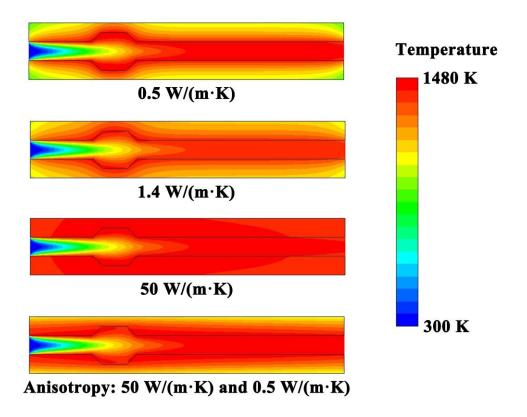
Figure 13. Contour plots of temperature at different thermal conductivities. The thermal conductivity of the anisotropic solid material is  $50 \text{ W/(m\cdot K)}$  in the longitudinal direction and  $0.5 \text{ W/(m\cdot K)}$  in the transverse direction.
