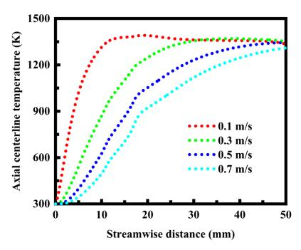
**Figure 8.** Axial fluid centerline temperature profiles along the length of the cavity-stabilized burner under different admixture inlet velocity conditions.
