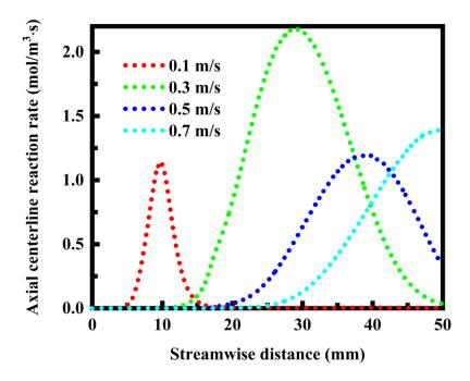
**Figure 10.** Axial centerline rate profiles of the combustion reaction in the cavity-stabilized burner under different admixture inlet velocity conditions.
