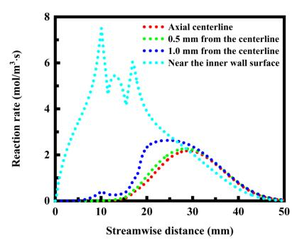
**Figure 11.** Transverse rate profiles of the combustion reaction at different distances from the axial centerline. The admixture inlet velocity is 0.3 m/s.
