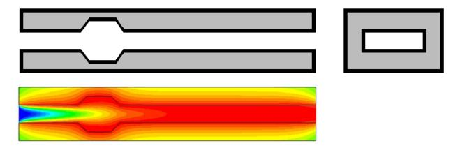
**Figure 1.** Schematic illustration of the millimeter-scale combustion system designed with cavities on the channel walls.
