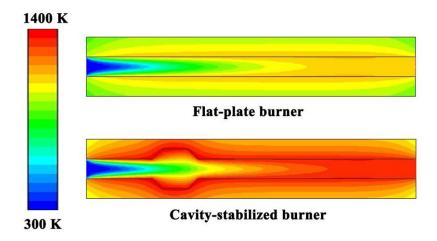
**Figure 7.** Contour plots of temperature for the flat-plate and cavity-stabilized burners. At room temperature, the thermal conductivity of the burner walls is 1.4 W/(m·K).
