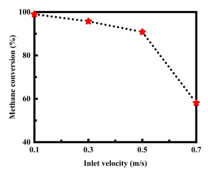
**Figure 9.** Effect of admixture inlet velocity on the methane conversion at the outlet of the cavity-stabilized burner.
