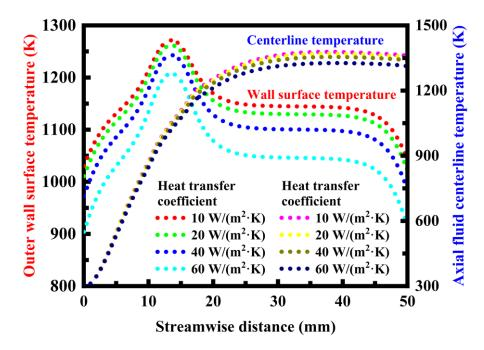
**Figure 16.** Temperature profiles along the outer wall surface of the burner and along the fluid centerline under different wall heat transfer coefficient conditions.
