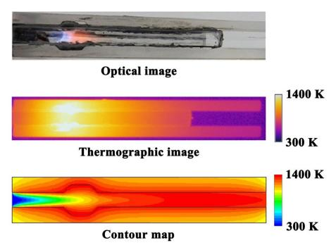
**Figure 4.** Laminar premixed methane flames and temperature variation in the burner. A constant fuel-air stoichiometry is maintained in operation.
