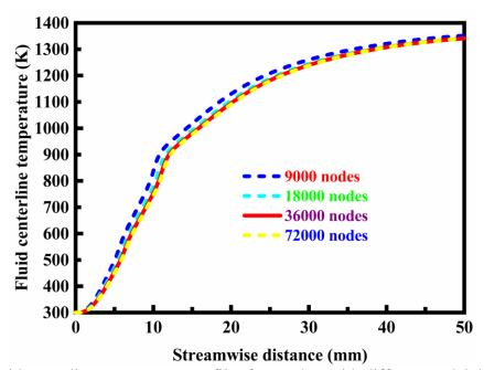
**Figure 3.** Fluid centerline temperature profiles for meshes with different nodal densities. The inlet velocity of the gases is 0.6 m/s, with a stoichiometric fuel-air ratio.
