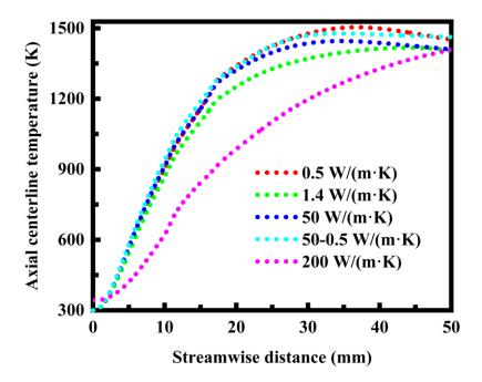
**Figure 15.** Temperature profiles along the fluid centerline of the cavity-stabilized burner under different thermal conductivity conditions.
