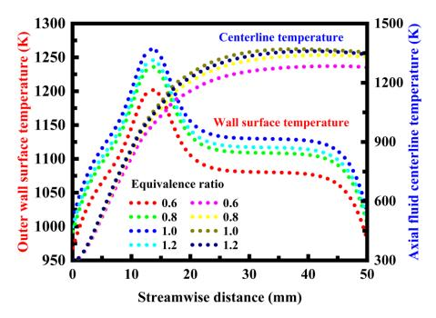
**Figure 18.** Temperature profiles along the outer wall surface of the burner and along the fluid centerline under different wall heat transfer coefficient conditions.
