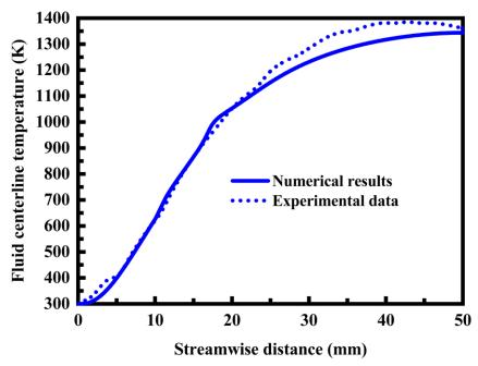
**Figure 5.** Fluid centerline temperature profiles determined from thermographic measurements and predicted by the model. A constant fuel-air stoichiometry is maintained in operation.
