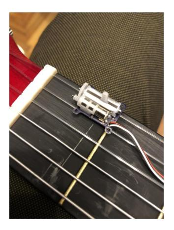
**Figure 13.** Linear servo-type motor on the standard classical guitar fretboard (Tolgahan Çoğulu, Personal Archive)
