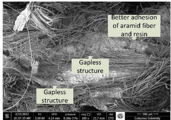
Figure 25 AP composites SEM micrograph
