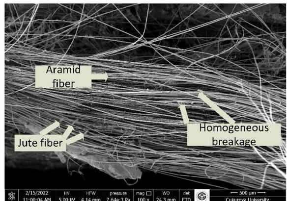
Figure 26 JAP hybrid composites SEM micrograph
