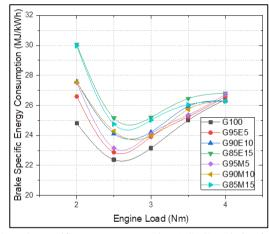
Fig. 4. Brake specific energy consumption (BSEC) variation for all test fuels at different engine loads
