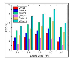
Fig. 9. EGT variations of all blended fuels compared to gasoline for different load conditions
