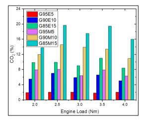
Fig. 13. CO<sub>2</sub> variations of all blended fuels compared to gasoline for different load conditions
