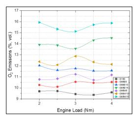
Fig. 10. O2 variation for all test fuels at different engine loads
