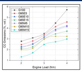
Fig. 14. CO variation for all test fuels at different engine loads
