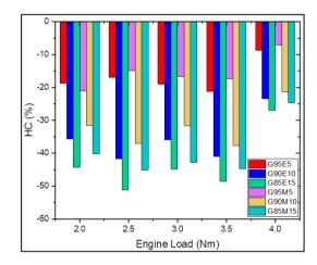
Fig. 17. HC variations of all blended fuels compared to gasoline for different load conditions
