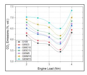
Fig. 12. CO2 variation for all test fuels at different engine loads
