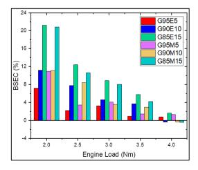
Fig. 5. BSEC variations of all blended fuels compared to gasoline for different load conditions
