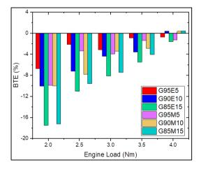
Fig. 7. BTE variations of all blended fuels compared to gasoline for different load conditions
