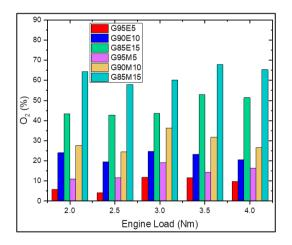
Fig. 11. O<sub>2</sub> variations of all blended fuels compared to gasoline for different load conditions
