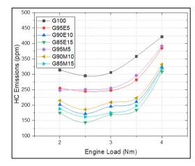
Fig. 16. HC variation for all test fuels at different engine loads
