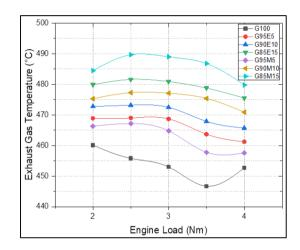
Fig. 8. Exhaust gas temperature (EGT) variation for all test fuels at different engine loads
