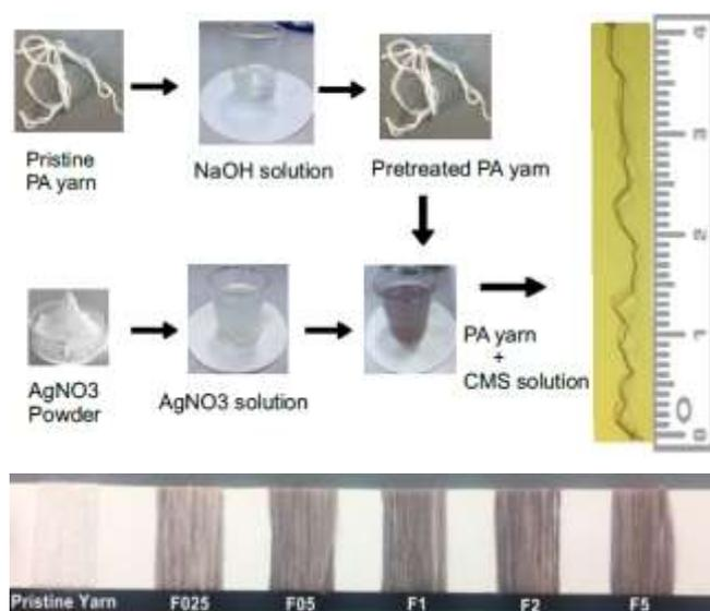
Figure 1. Preparation of AgNPs coated composite PA yarn
