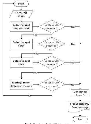
Fig.1. The flow chart of the system.
