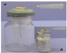
Figure 1. The experimental model used to evaluate debris extrusion during root canal retreatment.(a) Vial holding the device during instrumentation. (b) Vial covered with aluminum leaf to prevent the operator from viewing debris extrusion during the retreatment phase.
