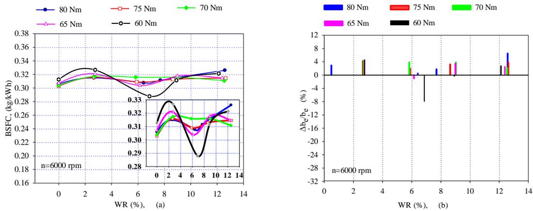
Figure 6 (a-b). Variations and VRs of BSFC versus different WRs under five different loads at 6000 rpm, respectively
