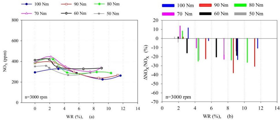
**Figure 11 (a-b).** Variations and VRs of NO<sub>x</sub> emissions versus different WRs under five different loads at 3000 rpm, respectively.
