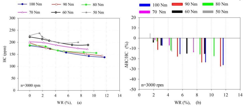
**Figure 15 (a-b).** Variations and VRs of HC emissions versus different WRs under five different loads at 3000 rpm, respectively.
