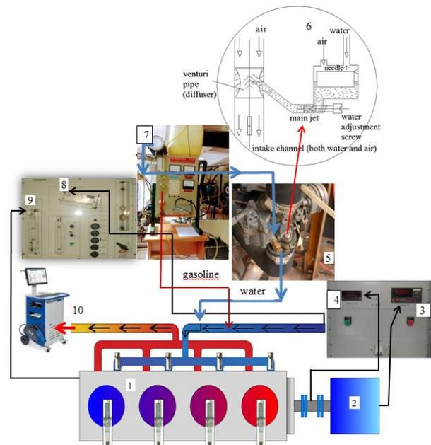
**Figure 1.** Experimental system. 1-Engine (Renault Clio), 2-Load unit, 3-Torque, 4- Engine speed, 5- Adapted carburettor, 6- Technical drawing of the adapted carburettor, 7- Water tank, 8- Air measurement manometer, 9- Coolant flow meter, 10- Exhaust gas analyzer
