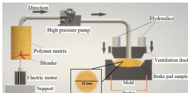
Figure 2. Illustration of sample preparation method
