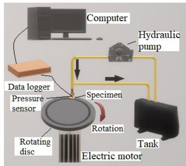
Figure 3. Schematic representation of the friction test rig
