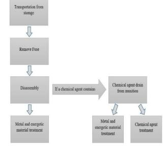
Figure 1. Disposal Process of Munitions
