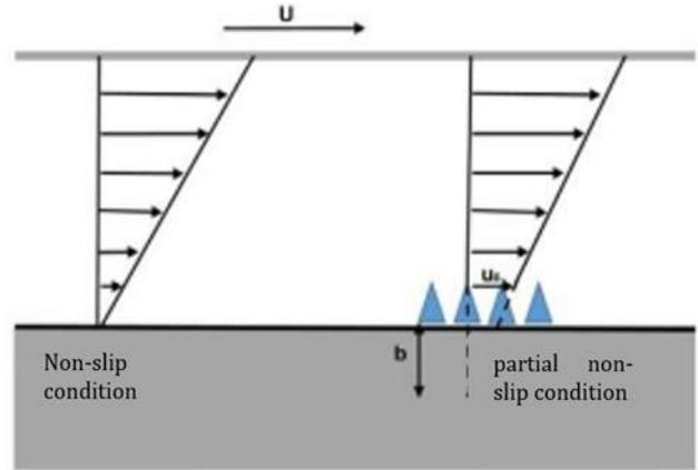
**Figure 10.** Effect of hydrophobic property on velocity profile [33].
