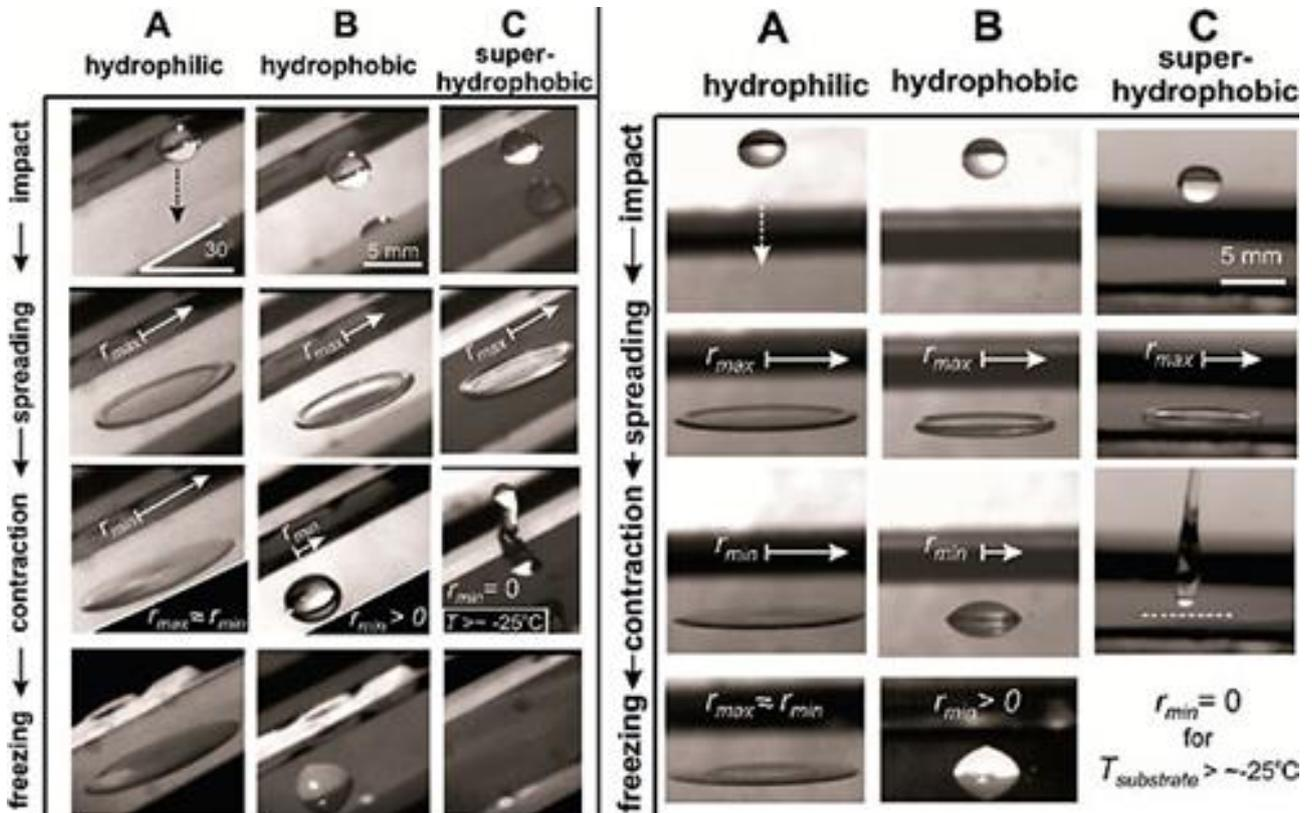
**Figure 8.** Dynamics of droplet behavior on hydrophilic, hydrophobic and superhydrophobic surfaces placed at an angle of 30° (left) and horizontal (right). The temperature of all surfaces is below zero. Drop temperature 0°C. The top-down photos describe the collision of the drop, the moment of maximum expansion ( $r_{max}$ ), followed by compression ( $r_{min}$ ), and freezing. For superhydrophobic surfaces, the compression radius is zero if its temperature is above minus 25 - minus 30°C [29].
