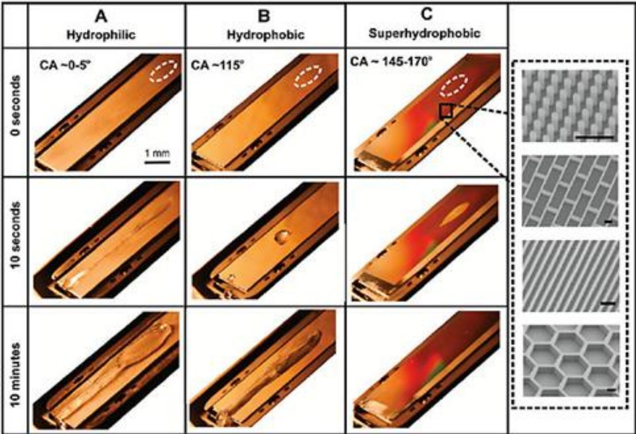
**Figure 7.** Ice accumulation on flat aluminum (A), smooth fluorinated Si (B), and microstructured fluorinated Si (C) surfaces. The advancing contact angle (CA) of the water droplets on these surfaces is indicated [29].
