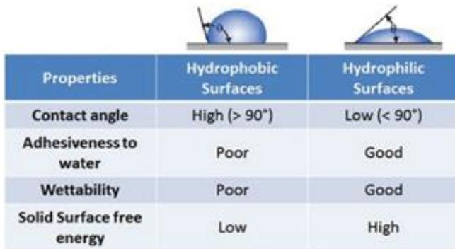
Figure 1. Hydrophilic and hydrophobic surface properties [5].
