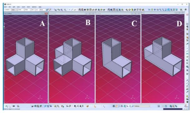
Figure 1. Four different connector designs
