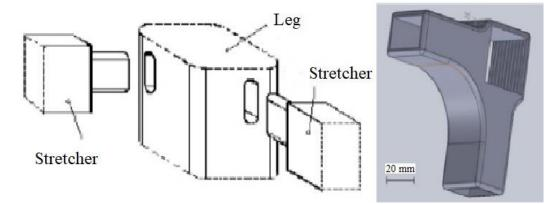
Figure 6. Mortise-tenon jointed chair leg and connector design for leg and stretcher (Nicolau et al. 2022)
