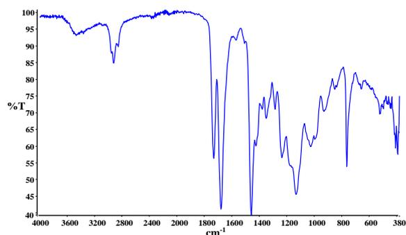
Figure 4. FTIR spectrum of PEI modified TE-APCR films.
