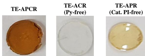
Figure 2. Digital photographs of the photocured discs.
