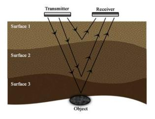
Figure 1. General working principle of GPR.
