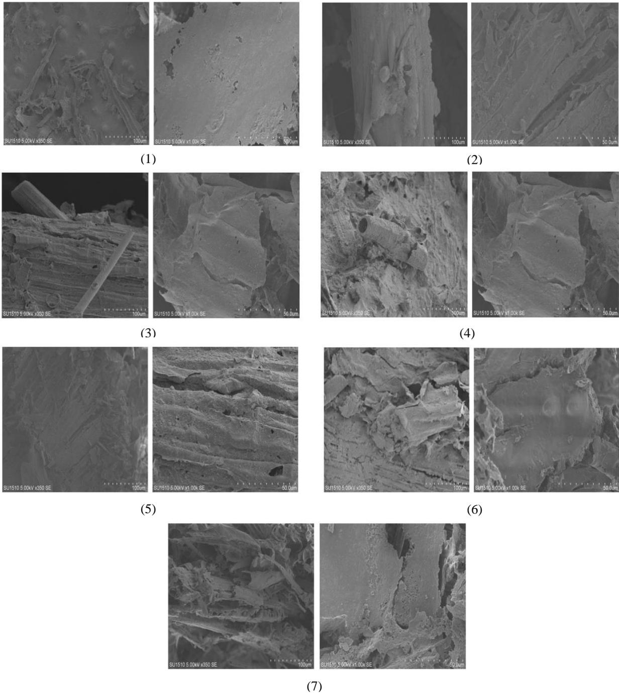
**Fig 4.** SEM images of organic matter untreated and ultrasonic pretreatment, (1) untreated, (2) 0.1 W/mL and 30 min pretreatment, (3) 0.5 kJ and 60 min pretreatment, (4) 1.0 W/mL and 20 min pretreatment, (5) 3.0 W/mL and 20 min pretreatment, (6) 5.0 W/mL and 30 min pretreatment, (7) 10.0 W/mL and 20 min pretreatment.
