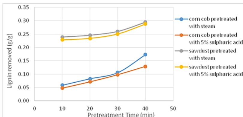
**Figure 5.** Estimation of lignin removed during pre-treatments
