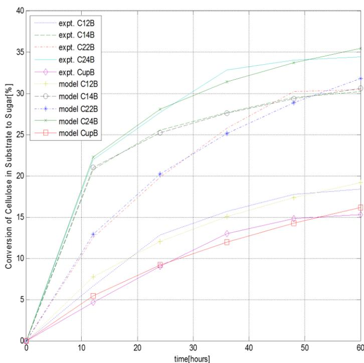
**Figure 9.** Comparison between experimental data and model output for sawdust samples hydrolysed with mixture of cellulase and  $\beta$ -glucosidase
