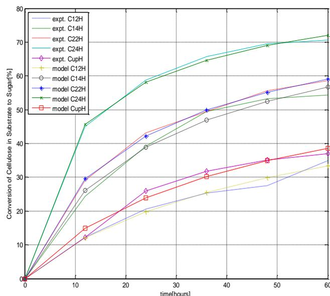
**Figure 6.** Comparison between experimental data and model output for corncob samples hydrolysed with mixture of cellulase and hemicellulase
