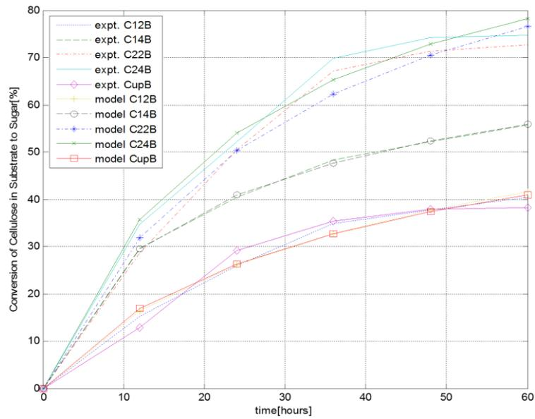
**Figure 7.** Comparison between experimental data and model output for corn cob samples hydrolysed with mixture of cellulase and  $\beta$ -glucosidase
