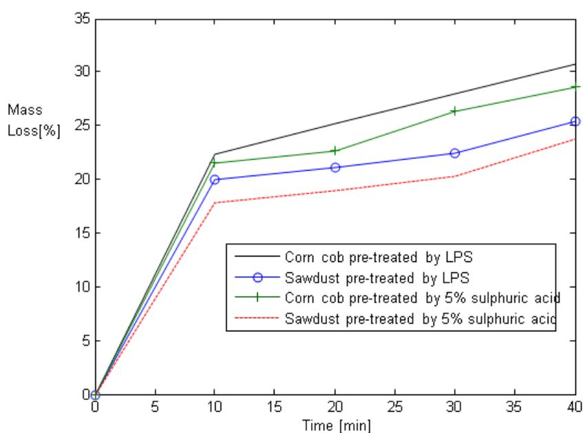
**Figure 1.** Loss of mass in pre-treated samples
