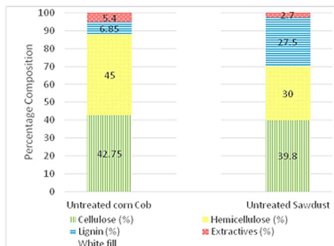
Figure 3. Chemical composition of untreated corn cob and sawdust
