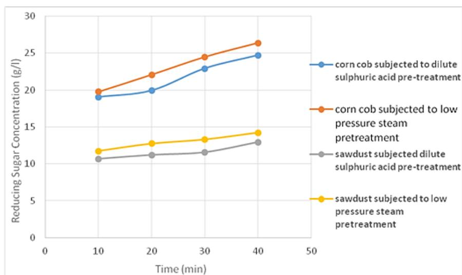
**Figure 2.** Effect of time on the RS present in prehydrolysate of both materials after 5% sulphuric and low pressure steam re-treatments
