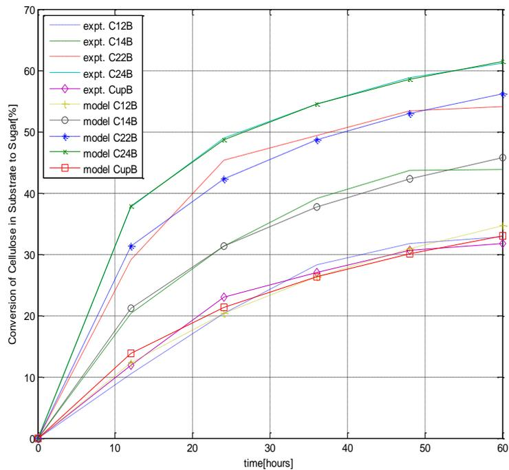
**Figure 8.** Comparison between experimental data and model output for sawdust samples hydrolysed with mixture of cellulase and hemicellulase
