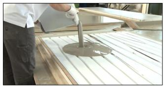
Figure 16. Pouring silicone & hardening component
