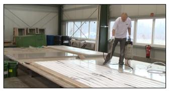
Figure 13. Warnishing mold release agent
