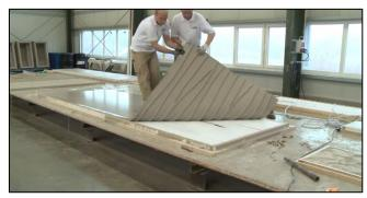
Figure 19. Removing silicone from molds
