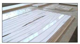
Figure 14. The model which warnished and ready for pouring silicone
