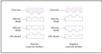
Figure 8. Concrete-Silicone Mold-CNC Model relations
