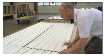
Figure 11. Interconnecting printed pattern pieces together
