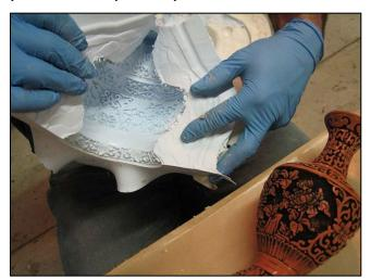
Figure 7. Silicone molding method in restoration application
