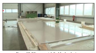
Figure 18. Silicone cast, lefted for hardening After enough hardening, silicone is removed from molds in the form of rolls and laid on the cutting area.
