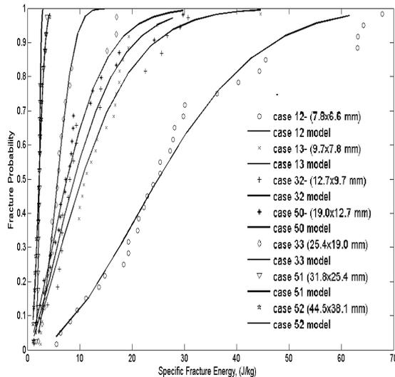
**Figure 6.** Weibull model fits to the experimental mass specific fracture energy data of all seven particle sizes [3]
