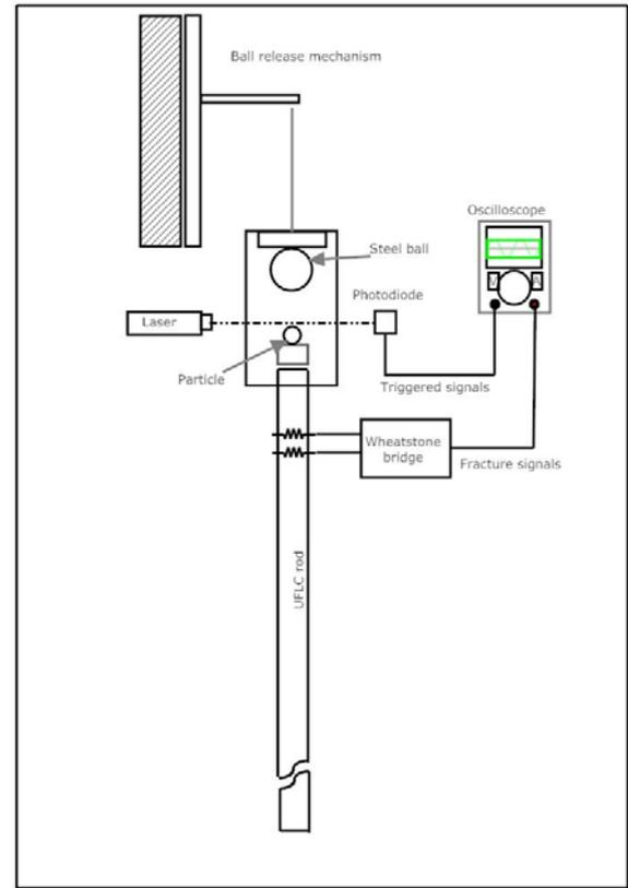
Figure 1. Schematic drawing of UFLC [3]
