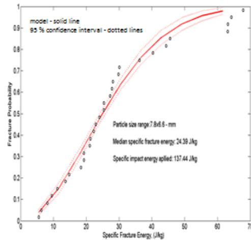
**Figure 5.** Weibull model fit to the experimental mass specific fracture energy data of 7.8x6.6 mm particle size
