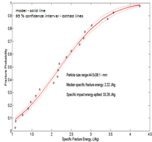
**Figure 4.** Weibull model fit to the experimental mass specific fracture energy data of 44.5x38.1 mm particle size
