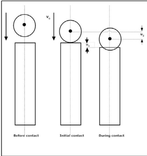
**Figure 2.** Deformations occurring in the UFLC rod and the falling sphere (deformations are measured from the center of the bodies)
