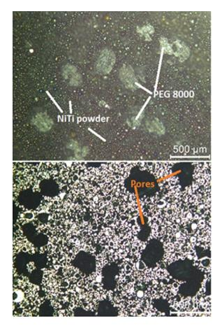
Figure 1. (a) Optical microscope image of the raw sample before the debinding process, (b) Optical microscope image of the sample sintered in Ar atmosphere at 1125 C for 1 hour
