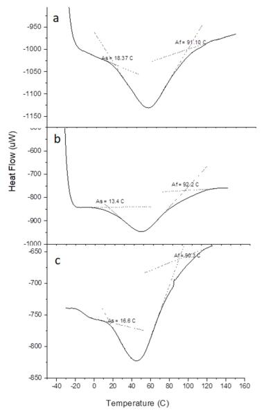
Figure 5. DSC curves of samples during heating (a) 1050 C, (b) 1125 C and (c) 1200 C
