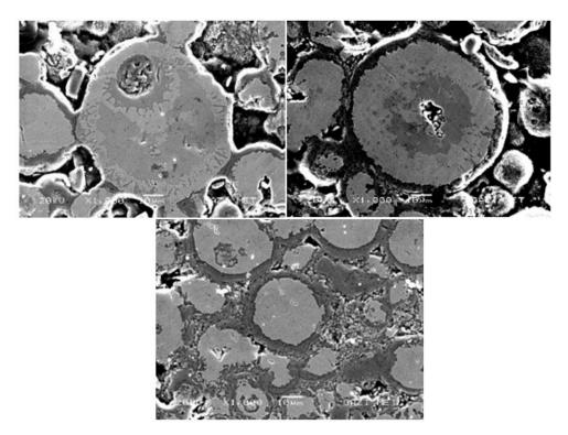
Figure 2. SEM micrograph of NiTi samples sintered for 1 hour a) 1050 C, b) 1125 C c) 1200 C
