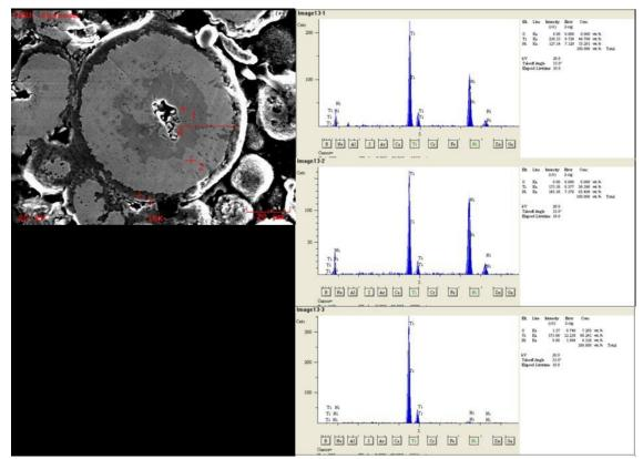
Figure 3. Point EDS analysis of the sample sintered in 1125 C 1 hour Ar atmosphere
