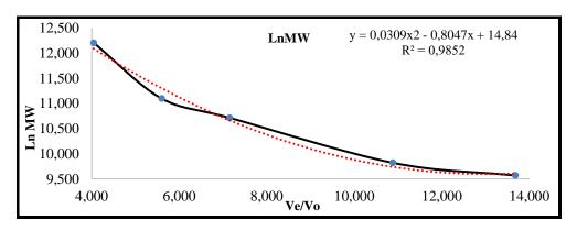
Figure 4. Gel filtration chromatography standard curve
