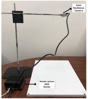
Figure 6: The experimental setup
