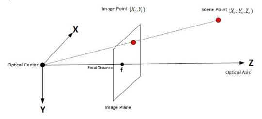
Figure 5: Transition from picture coordinate system to camera coordinate system.
