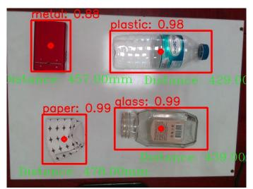
Figure 7: Real-Time Waste Detection
