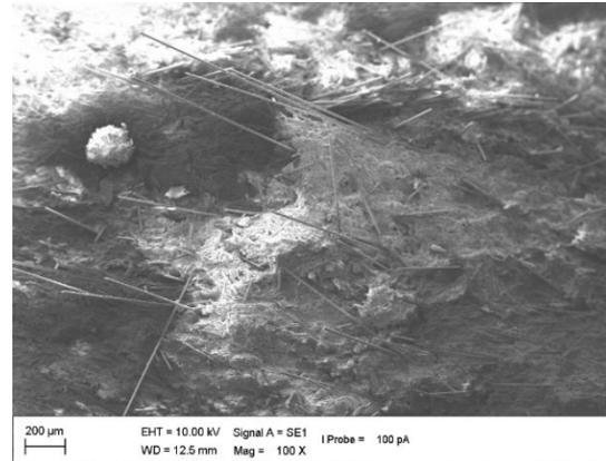
Figure 2. The SEM images of the fractured surface of reinforced WPCs with 5% glass fiber.
