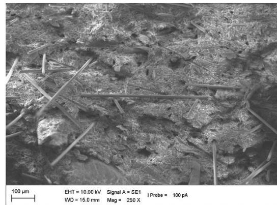
Figure 3. The SEM images of the fractured surface of reinforced WPCs with 15% glass fiber.
