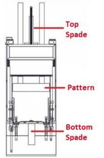
Fig. 1. Vulcanization press working principal diagram
