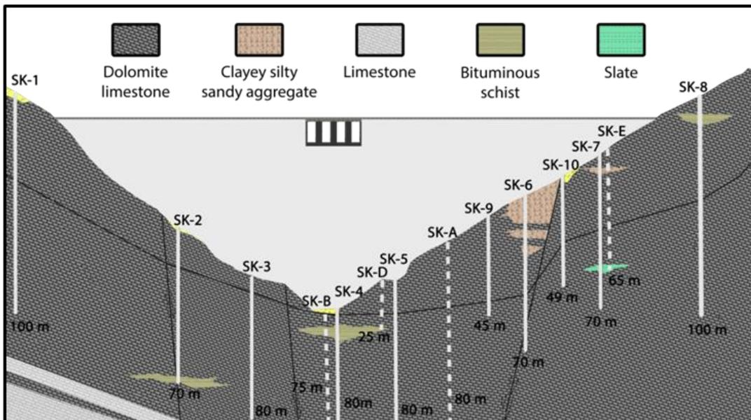
Figure 3. Geological profile of the dam foundation.
