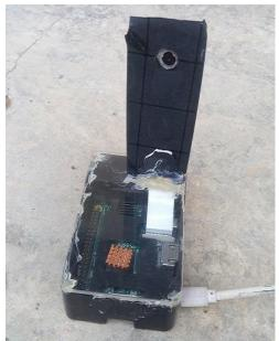
Fig. 7. Prototype of intelligent surveillance system using Faster RCNN
