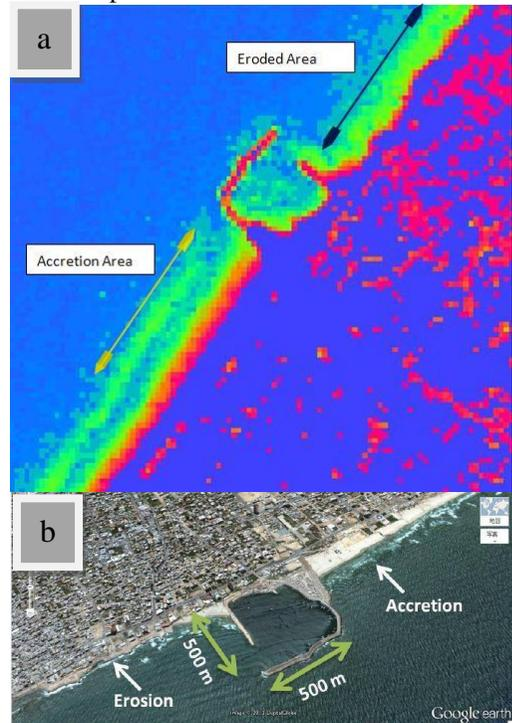
Fig. 10. a) TSS accumulation on one side and lacking on the other side of Gaza seaport. b) Beach erosion and accretion around Gaza seaport as a result to TSS disturbance in distribution around the seaport.
