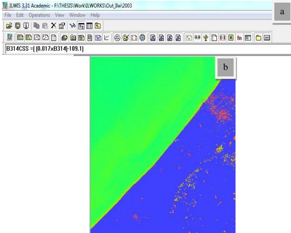
Fig. 6. a) Illustrates the used code in ILWIS command window for TSS concentrations calculations. b) Resulted TSS map from the used equation ( $TSS = 0.017DN - 109.1$ ) as an example.
